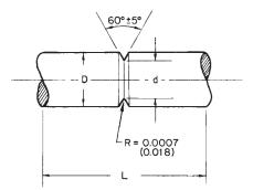
NOTE 1—Dimensions are in inches and (millimetres). NOTE 2— d must be concentric with D within 0.025 mm (0.001 in.).
